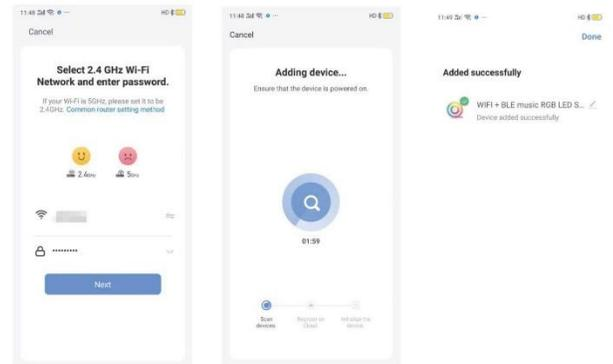
Step 3 . Confirm that the 360° Return Smart Light is flashing quickly-enter the Wi-Fi password to connect with the light ,connection successful . Choose the light level, color, and scene you like.
