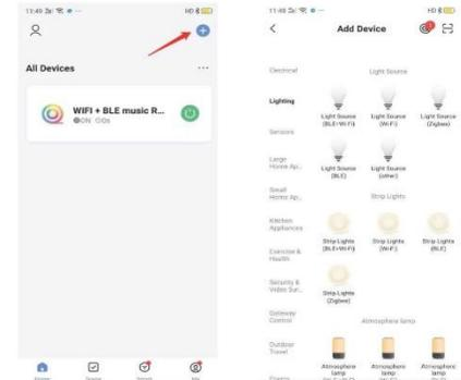
Step 2. Follow the instructions on the APP and let your device enter setup mode. If the light is blinking fast, skip the reset step
